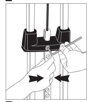
Once the Selector Stem is centered, retighten the socket cap bolt securely.
